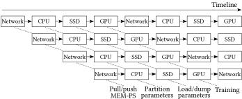
Figure 7. The 4-stage pipeline.
