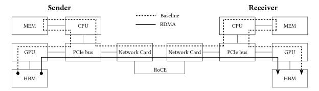
Figure 8. Inter-node RDMA communication.
