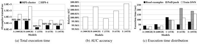
Figure 3. The performance (execution time and accuracy of 4-node hierarchical parameter server (HPS-4).
