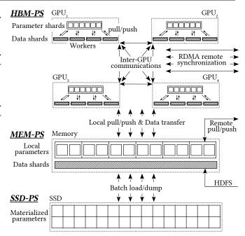
Figure 2. Hierarchical parameter server architecture.
