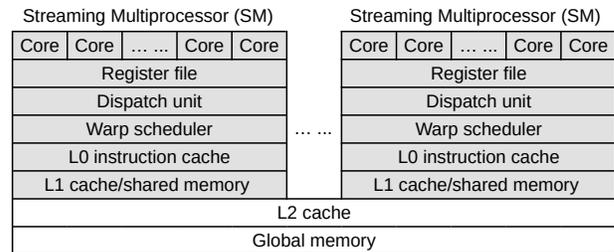
Fig. 2: GPU architecture.
