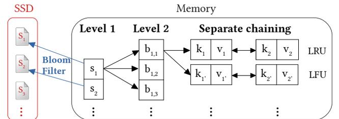
Figure 4: The architecture of the bi-level cache management.
