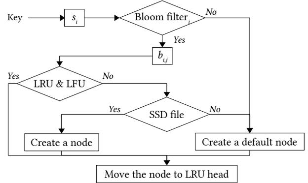
Figure 5: The workflow of the Sparse Table pull operator.
