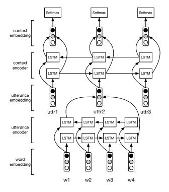
Figure 1: *Hierarchical Bi-Directional LSTMs model architecture.*
