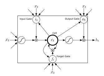
Figure 2: Long Short-Term Memory Unit Structure.
